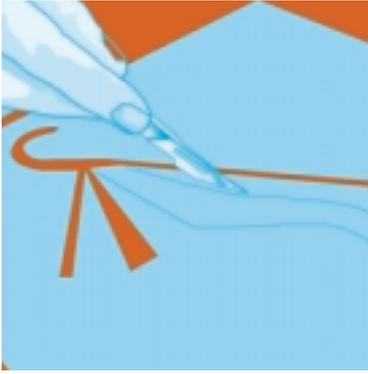
1. Place the stencil film matt side up and cut into the top layer with a scalpel to make the design, leaving the transparent backing film intact.
