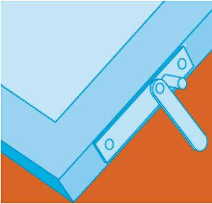
To help in removing a wet print and positioning substrate prior to printing, it is a good idea to make a prop bar for one side of the frame. This can be made from wood or metal about 10cm long, placed on the frame to allow it to stand at 45°.
