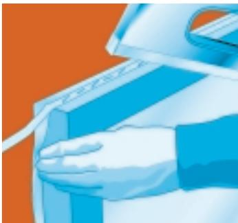
Cut the mesh to size, allowing an approximate 3cm overlap on each side of the frame. When attaching the fabric, staple through a thin strip of card to avoid tearing the mesh.
