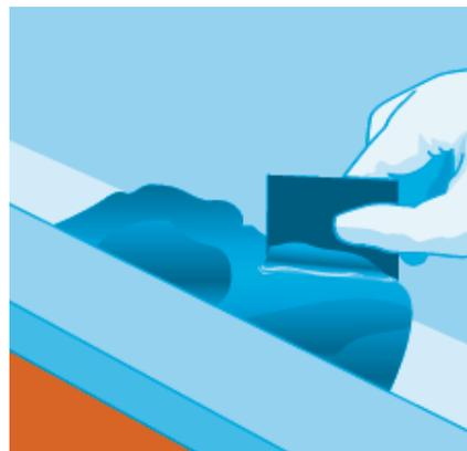
5. Use a piece of card to spread a coating of Xtend filler over bare areas of fabric around the stencil. When the filler is dry the screen is ready to print.
