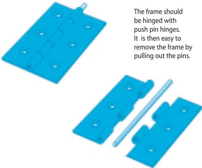
The frame should be hinged with push pin hinges. It is then easy to remove the frame by pulling out the pins.
