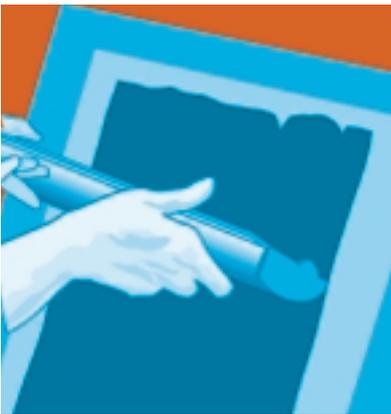
1. Fill a coating trough with light-sensitive emulsion. Draw the trough up the screen at an angle to lay an even coating of emulsion on the mesh.
