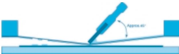
The screen mesh must on no account come into contact with the printing paper when the frame is laid down upon it prior to printing. There should be a gap of about 0.5cm between the mesh and the paper. Generally the only exception to this rule would be when printing fleece fabrics.
