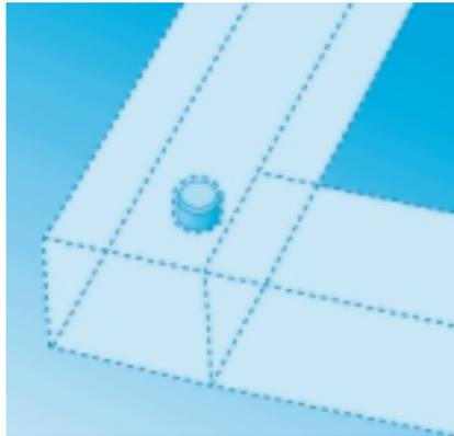
To minimise any lateral movement in the frame and to ensure correct registration, fix a short dowel into the baseboard, protruding about 5mm. Drill a hole in the underside of the frame so that when it is lowered for printing the dowel interlocks.
