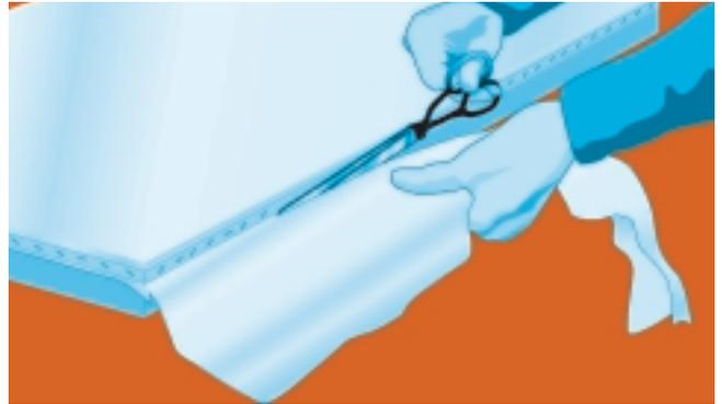
Use scissors or a sharp knife to trim off any surplus mesh around the edges of the frame.
