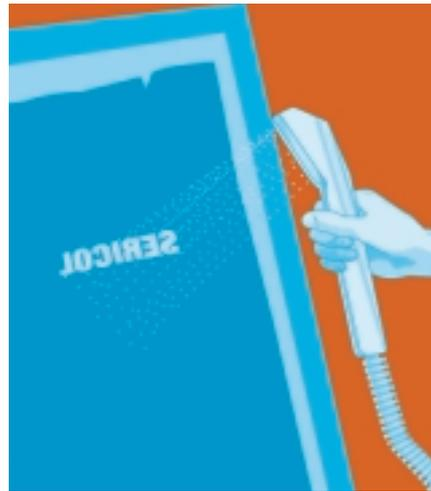
4. After exposure, wash the screen out with water. The emulsion has been hardened by the light but those areas protected by the positive image are washed away.
