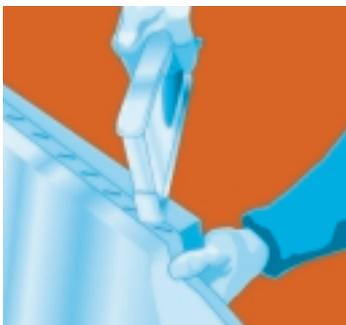
Staple from the centre of one side of the screen towards each corner, pulling the fabric tight as you work. Put the staples at an angle across the side of the frame.
