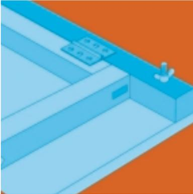
Fix the hingebar to the baseboard. A bolt and wing nut at each end of the bar enable it to be raised if necessary.
