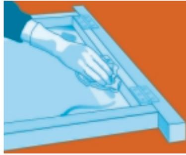
3. Wipe out the inside of screen and mesh with thinners and clean wipers. Rest the screen on sheets of newsprint and work until the mesh is quite clear of ink.
